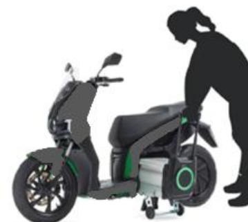
Transport and insert the battery pack into the scooter
