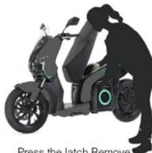
Press the latch Remove the battery pack
