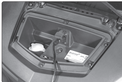
Fig. 130 - Vehicle connection point.
