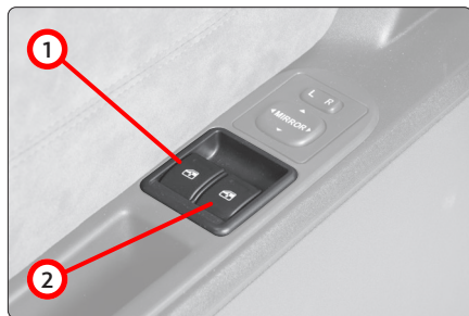
Fig. 108 - Close-up of driver's door: controls for windows.
