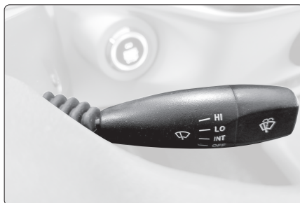
Fig. 117 – Wiper lever in the Único version.
