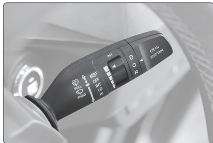
Fig. 116 – Windscreen control - Located to the right of the wheel.
