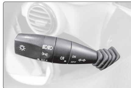
Fig. 113 - Turn signal and high beam lever on Unico version.
