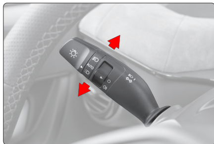
Fig. 28 - Light control - Located to the left behind the wheel.
