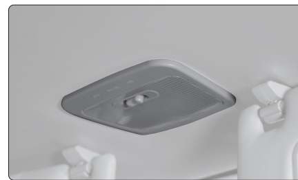
Fig. 115 - Courtesy light on roof.
