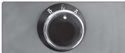
Fig. 32 - Gear selector - Centrally located above the console.
